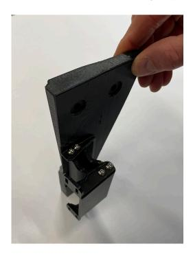
Please note orientation of parts. Dome head machine screws.
