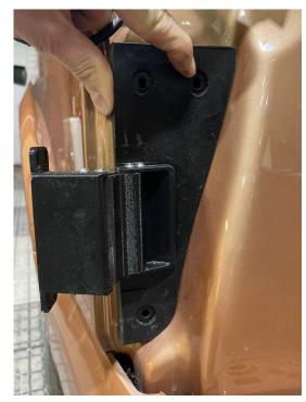
Place and hold your main hinge panel in place. To get this panel in the correct area locate the right hand side tight against the body work. Please see picture for reference.
