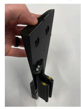
Please see correct hinge layout. Note the indentations on top outer edge (marked in yellow for this example). Dont over tighten as hinges need to move freely. Add 2 screws top and bottom. Dome head machine screw.
