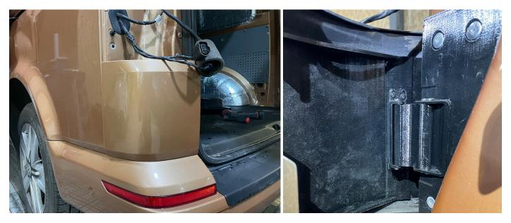
Place flap onto vehicle and gap correctly using body swage lines. Once you are happy with the placement open up the flap and mark hinge location. Spot drill holes for hinge fixings. Use No6 1/4 flanged black screws top and bottom to fix hinge to door.
