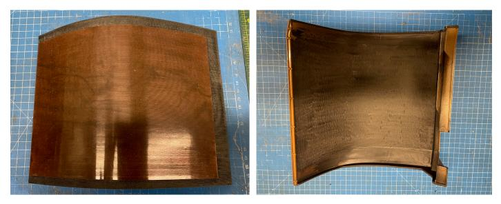
Clean all plastic surfaces before applying any adhesive. Clean back of 3d printed flap seen in image 1. Then clean inside of OEM panel. Once cleaned apply double sided glue sheet to back of 3d printed panel as seen in image 1.
