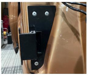
We recommend applying some silicon or mastic around the holes before securing with the rivets. Use 3 peel rivets (supplied) to secure the panel.
