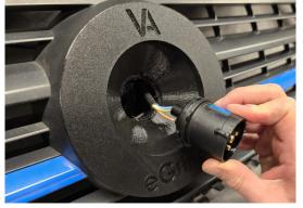
Run your 240v 3-core cable to the grill cutout, ensure the grommet is installed into the e-grille and push the cable through
