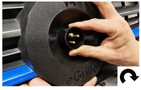
**NOTE:** ONCE INSTALLED YOU NEED TO GAIN ACCESS TO THE REAR OF THE EGRILLE TO REMOVE.
