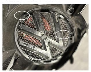
You will need to use the trim tools to remove the grille from the front of the vehicle. Once removed use trim tools or a small flat screw driver to remove the existing badge by unclipping and rotating the badge to
