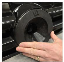
Insert the eGrille in the correct orientation and lay the grille on its face.
