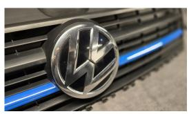
To install the badge adapter, align the plug to the adapter at approx. 2oclock and push in until flat with the grille.
